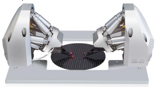
Hexapod micro-positioner x-y resolution 100 nm; z resolution 50nm
